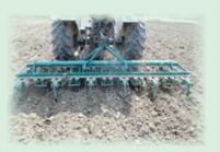
helps in pulverize the soil at the deeper layer means up to 15-20 cm of soil depth.
